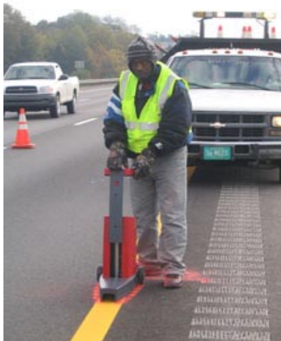
UT graduate student Godswill Nsofor takes retroreflectivity readings on the yellow edge line of Interstate 40 near Knoxville.
