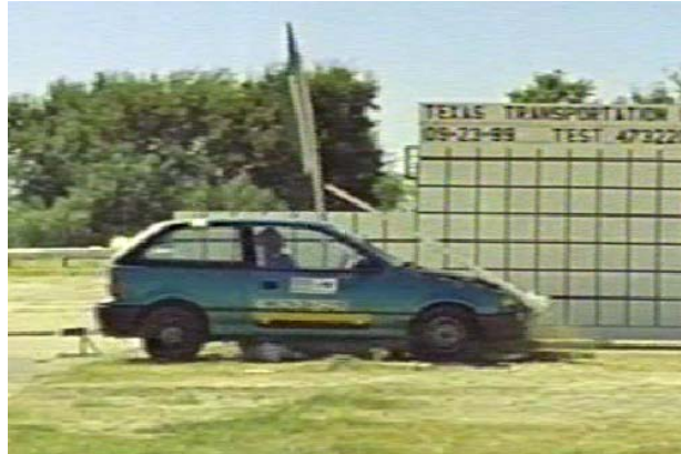
Crash-testing a work zone device (TTI).
